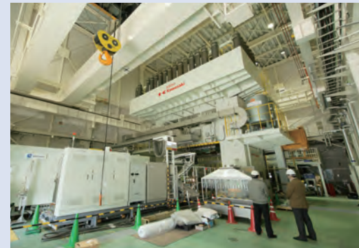
大物LFT-D高速成形システム Large LFT-D (Long Fiber Thermoplastic - Direct) high speed forming system
