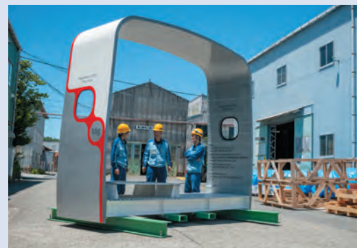
難燃性マグネシウム合金製高速鉄道車両試作構体 Prototype of high-speed railway car body made from flame-retardant Mg alloy
